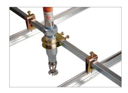
Connect sprinkler head to the reducer. Apply an un-aerobic pipe joint compound or Teflon taps to the NPT male threads of the sprinkler head according to the sprinkler head manufacture's instruction. Conduct pressure test
